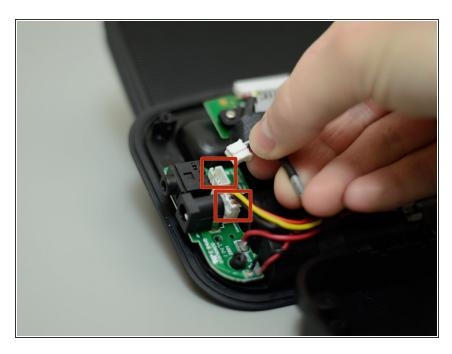
Firmly and cautiously unplug the two white 3-pin connectors from the printed circuit board.
