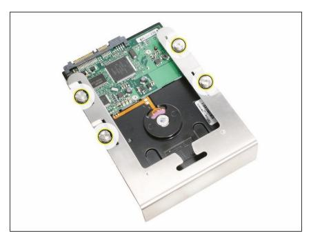
If you are replacing the hard drive with a new drive, remove the four screws that mount the 3, drive to the
