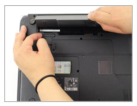
Slide the horizontal latch to the right to pop open the battery pack.
