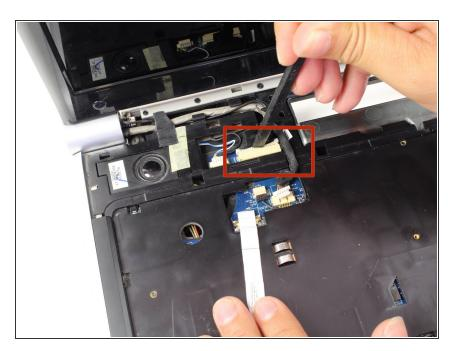
Using the flat edge of the spudger, disconnect the big white LCD cable connector by slightly pulling on it until it's detached from its respective port.
