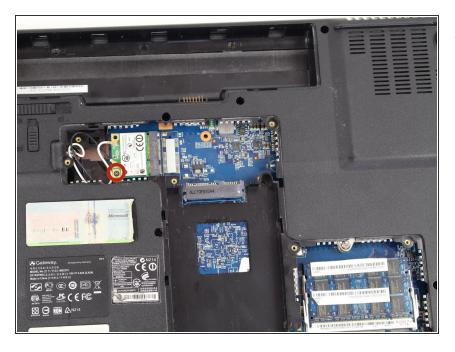
Remove the 3/16" Phillips #0 screw located at the bottom left corner of the WiFi card.
