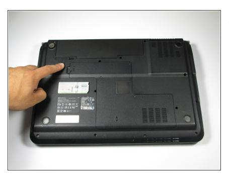
In order to unlock the battery, slide the vertical latch downward where it indicates the unlocking icon.
