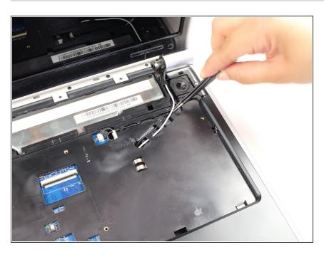
Using the tweezers, pull out the black and white cables located at the right side of the laptop.
