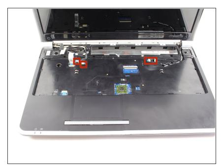
Locate the three LCD connectors.
