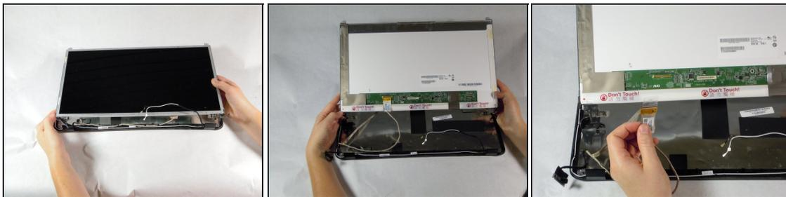
⚠ Be careful when moving the screen, you may damage the monitor and webcam cable.
