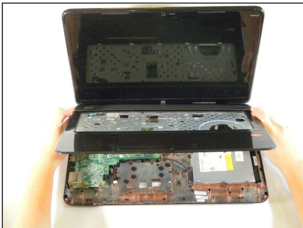
⚠ **Lifting the top panel too quickly or forcefully may damage the speaker cable, which is still attached underneath.**
