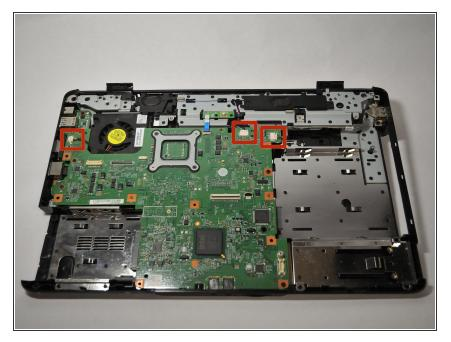
Disconnect the Thermal Fan cable,
