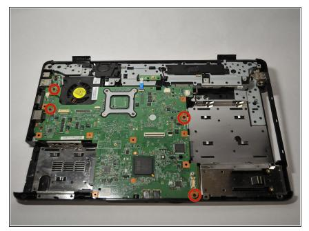
Remove the two screws (3mm, Phillips #1) on the left and the two screws (5mm, Phillips #1) on the right that secure the Motherboard to the laptop.
