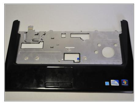
To separate the palm rest from the rest of the computer, use a plastic opening tool to lift up the plastic. It is best to start at one point and work your way around.
