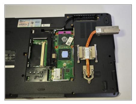
Pull up on the Heat Sink unit to remove it.
