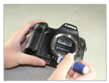
Remove the 8mm Phillips #00 screw from the bottom of the front of the camera.
