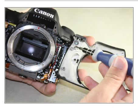
Remove the 4mm Phillips #00 screw on the inside of the front panel to separate the panel from the speaker wire.
