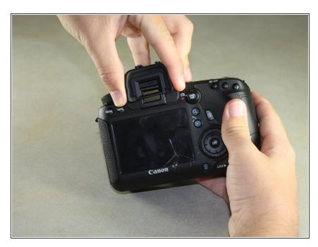
Remove the viewfinder cover by pinching the sides and sliding it upward.
