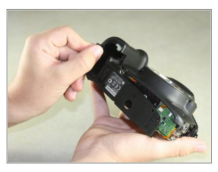
Remove the bottom panel from the camera by using your fingers to pull outward on the tab inside the battery compartment.
