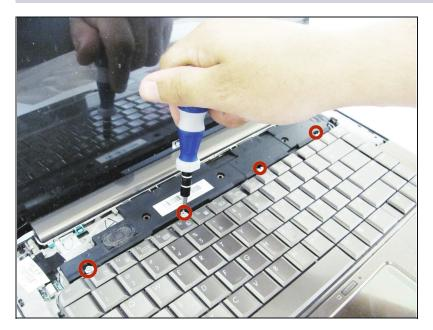
Use a <u>2.5mm flathead</u> screwdriver to remove the four 3mm screws on top of the keyboard.
