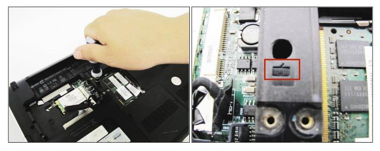
• Locate the hole in between the hard drive and RAM compartments.
