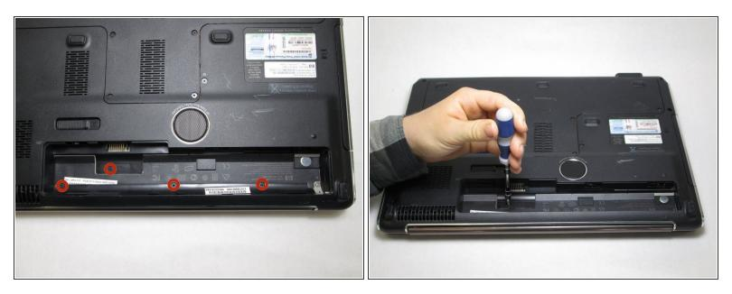
Using a Phillips Screwdriver, remove the four Phillips M25x3.0 head screws.
