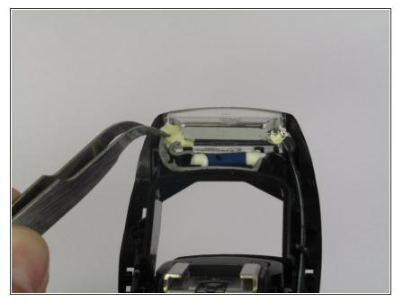
• Use the tweezers to remove the excess glue around the wiring. This will allow you to cut the wire and remove the light in the next step.
