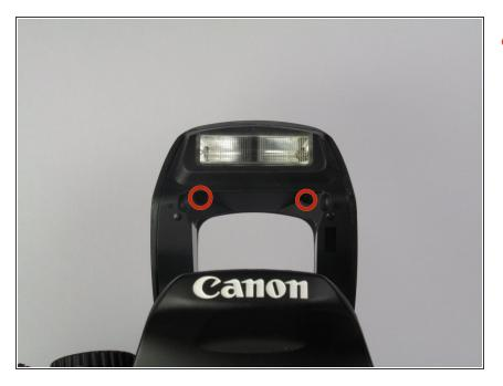
Using the Phillips screwdriver, unscrew the two 4.9mm Phillips head screws which are located underneath the flash.
