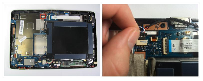
• Carefully remove the connector cable by pushing on the rim of black plastic insert.
