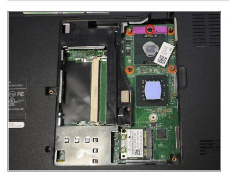
Using a flathead screwdriver, rotate the locking mechanism counterclockwise to the unlocked position.
