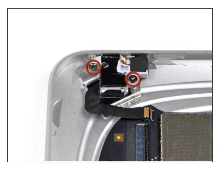
Remove the two 2.8 mm T5 Torx screws securing the headphone jack to the rear case.
