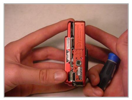
Gently detach the back cover by holding onto both sides of the camera and pulling them apart.
