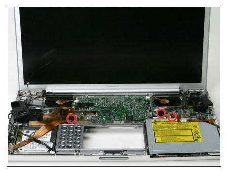
In order to disconnect the speaker cable from the front edge of the logic board, you must disconnect the sound cable, the optical drive cable, and the PRAM battery cable.
