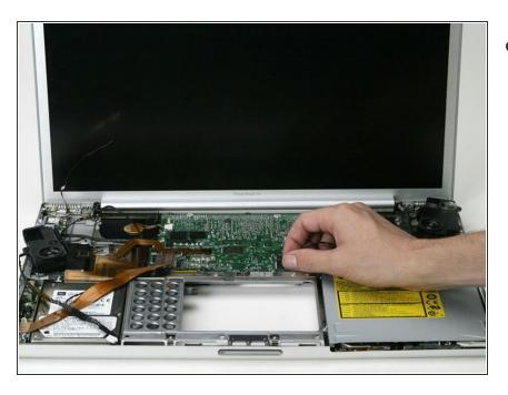
Deroute the speaker cable from the front edge of the logic board.
