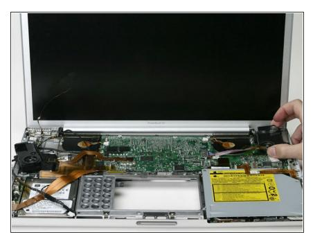
Deroute the display data cable from the left side of the speaker and pull the speaker assembly off the logic board.
