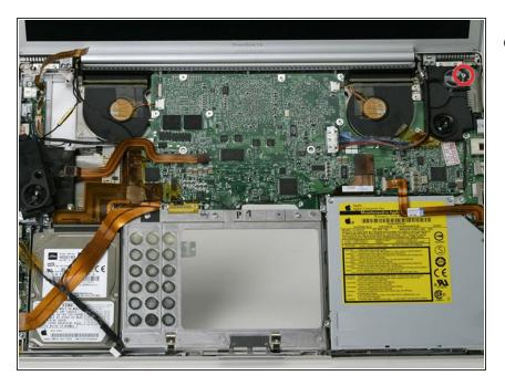
Remove the single T8 Torx screw from the right speaker assembly.
