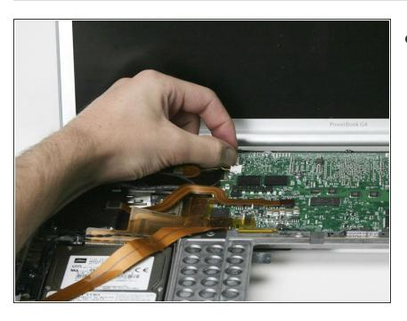
Disconnect the orange DC-In cable from the logic board.
