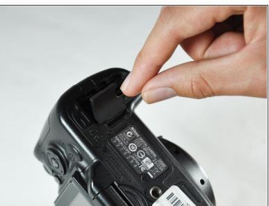
On the bottom of the camera, pull the release tab towards the center of the camera, then pull up.
