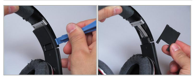
Use the plastic opening tool to gently pry the black plastic hinge piece directly away from the headband as shown.
