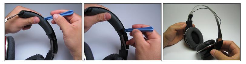
• Using the plastic opening tool, **gently** pry the headband cushion directly away from the plastic portion of the headband as shown. Pry the plastic portion a small amount and then move the opening tool sideways along on the headband. Repeat on both sides until the cushion separates from the top plastic part of the headband.
