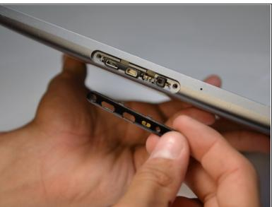
There are two 6.6 mm screws that hold ports into place as well as the back panel. Remove these with a T5 Torx screwdriver.
