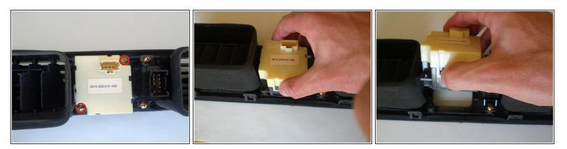
Remove two screws to remove the clock assembly.
