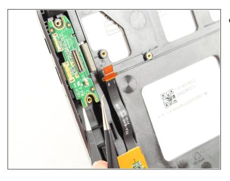
Once the screws are out, use the tweezers to pull the board straight out.
