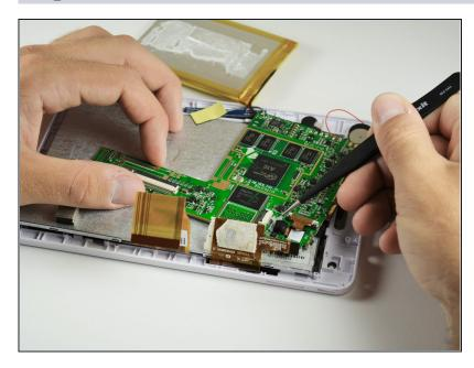
There may be hot glue holding down the front camera. Use the tweezers to carefully pull it off.
