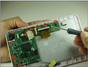
Use a Phillips #00 screwdriver to remove the eight 40mm screws holding the motherboard in place.
