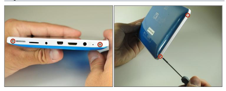
• Remove the four 30 mm Phillips #00 screws from the outer case.
