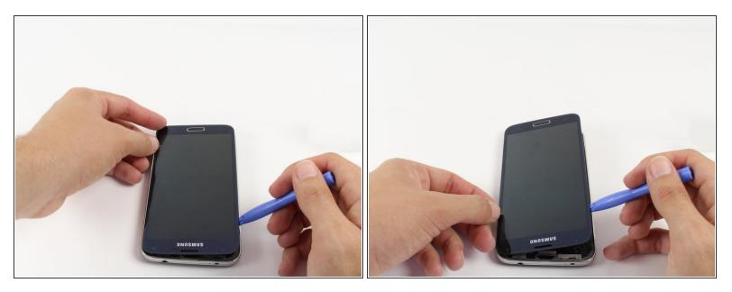
• Use a light amount of force when removing the screen.
