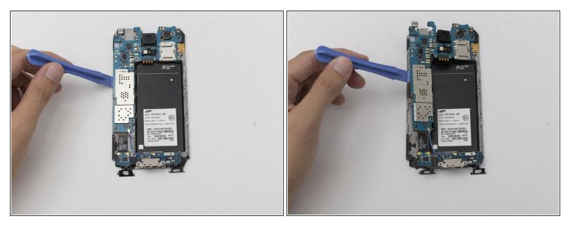
• Gently lift the motherboard off of the second midframe with the plastic opening tool.
