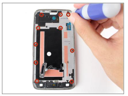
Unscrew the ten 4 mm screws from the midframe with a Phillips#00 head screw driver. You may want to use tweezers or a magnetic screwdriver to remove them.
