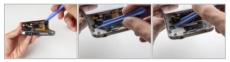
• Start lifting the screen from the top. You will see a black ribbon cable attaching the display to the motherboard. Use the plastic opening tool to lightly detach the connector.
