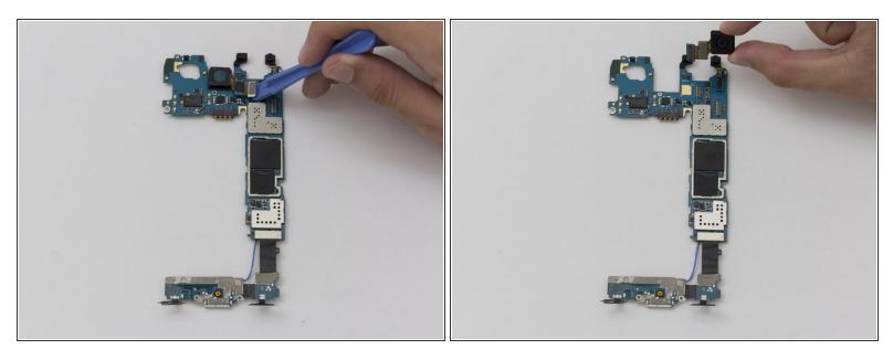
Use the plastic opening tool to gently remove the ribbon cable connecting the rear camera to the motherboard.
