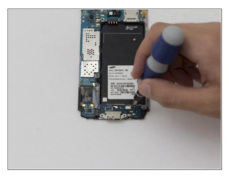
Remove the single black 4 mm screw from above the charging port with a Phillips#00 head screw driver.
