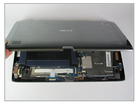
Once you have successfully pried the spudger in between the front case and back case, continue do so around the entire tablet until the back case is completely disconnected.
