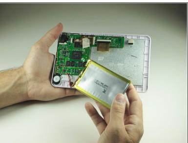
Use a plastic credit card, or other thin object, to separate the battery from the screen.
