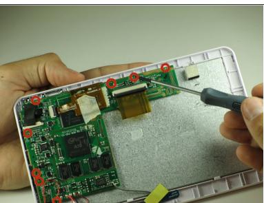
Use a Phillips #00 screwdriver to remove the eight 40mm screws holding the motherboard in place.
