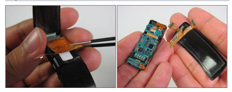
• Gently peel the screen assembly up and away from the device using tweezers.
