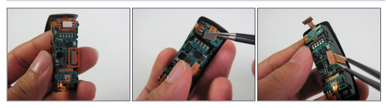
• Disconnect the ribbon cables connecting the screen to the motherboard by lifting their metal connectors up off of the board with tweezers.
