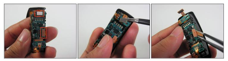
• Disconnect the ribbon cables connecting the screen to the motherboard by lifting their metal connectors up off of the board with tweezers.
