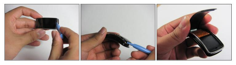
The screen is connected to the device by a ribbon cable on the left side with the power button facing you. Do not try to completely separate the screen from the device yet, and be careful.
