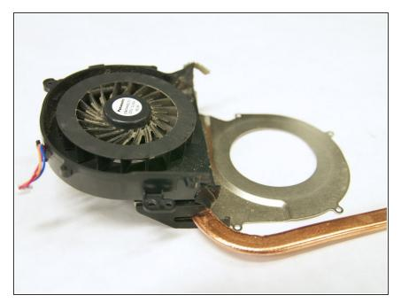
• The fan attached onto the heat sink with electrical tape. Removing the electrical tape allows you to replace the fan.
