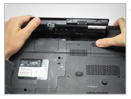
• With your thumb still holding the slider to the left, use the opposite hand to lift the battery out, removing it from the computer.
