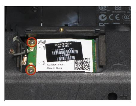
Remove the two 4mm screws with the Phillips #1 screw driver.
