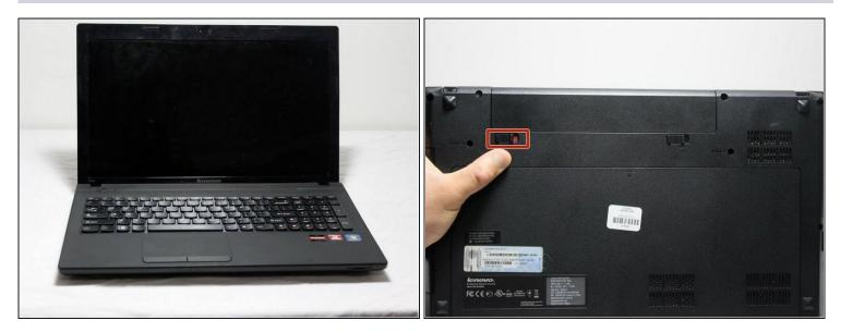
• To unlock the battery, flip the laptop over so that the bottom is facing upward. Then unlock the left clip by pushing the clip to the left.
