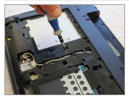
• Locate and remove the single screw right of the optical drive
