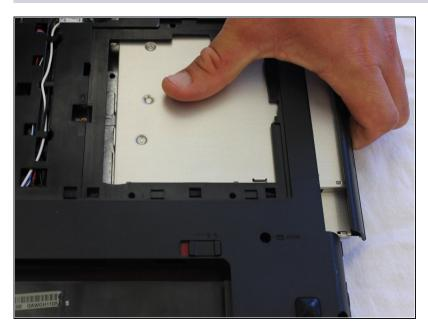
• Optical Drive should slide out easily with one thumb's effort.
