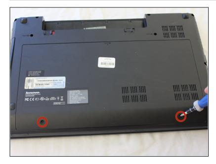
• Remove the two screws highlighted.
