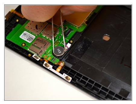
Remove the circular motor unit by gently pulling up on it using a tweezer.
