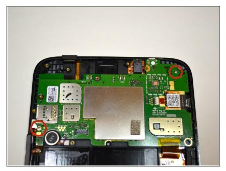
Using a #000 Phillips screwdriver, remove the two M1.4 3.5mm screws from the system board and set them aside.
