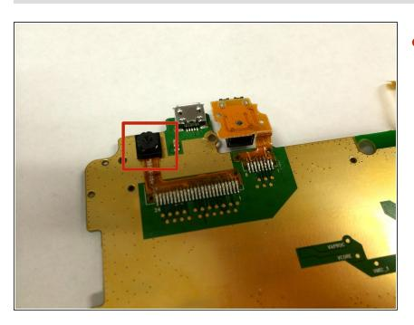
The camera is located on the backside of the system board.
