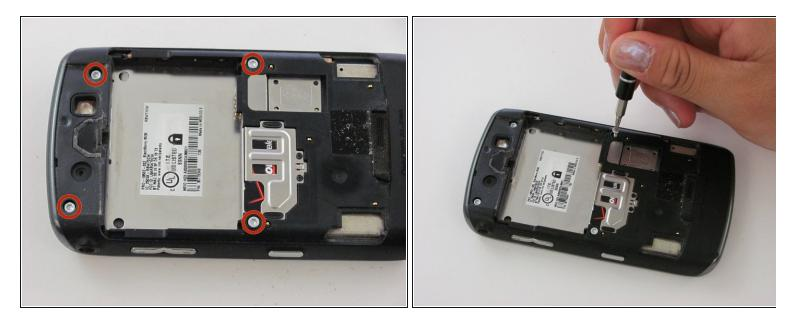
• Remove the four silver Torx T6 3 mm screws on the back of the device.
