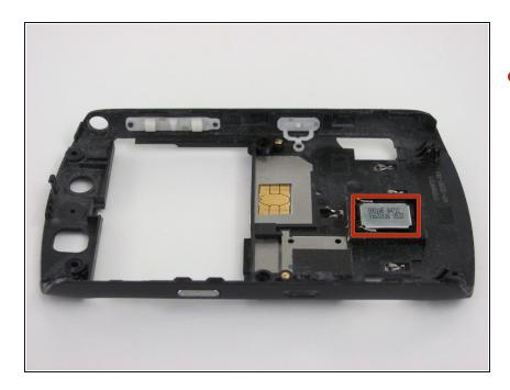
Locate the silver speaker marked with numbers and letters on the back panel of the device.
