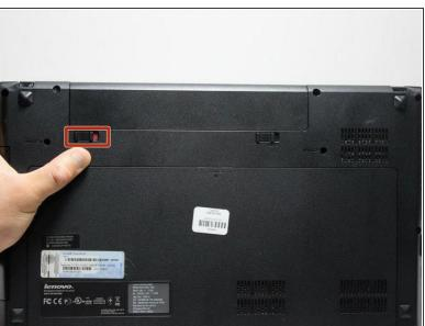
To unlock the battery, flip the laptop over so that the bottom is facing upward. Then unlock the left clip by pushing the clip to the left.
