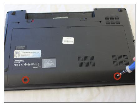
Remove the two screws highlighted.
