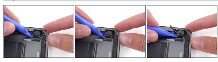
• Slide a plastic opening tool under the rear facing camera and pry upward to free it from the adhesive securing it to the rear case.
