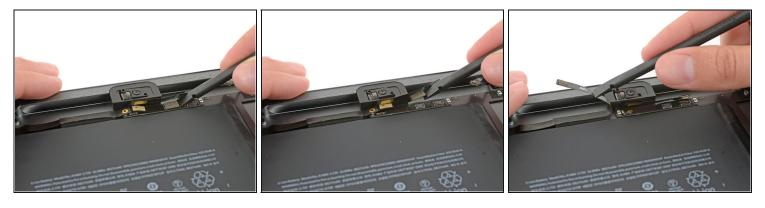
• Use the flat end of a spudger to disconnect the headphone jack connector from the logic board.
