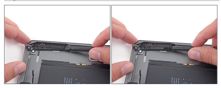
• Use the flat end of a spudger to pry in the gap made by the opening pick, lifting the bracket off of the adhesive.
