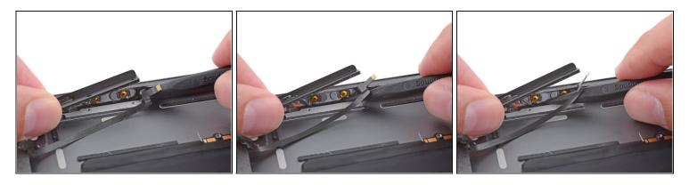
• Slide the point of a spudger under the ribbon cable near the button cables to free it from the adhesive holding it to the rear case.
