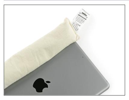
Place a heated iOpener on the upper left corner of the rear case to loosen the button bracket's adhesive.
