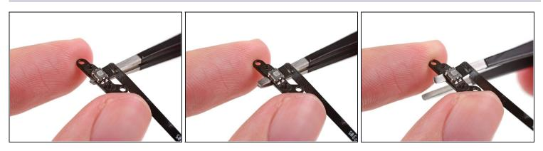
• Use one tine of a set of tweezers to pry the sleep/power button up from its bracket.
