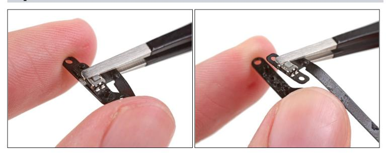
Remove the sleep/power button from the bracket.
