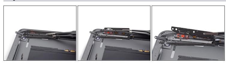
• With a set of tweezers, flip the front end of the button bracket up to allow access to the rest of the button ribbon cable.
