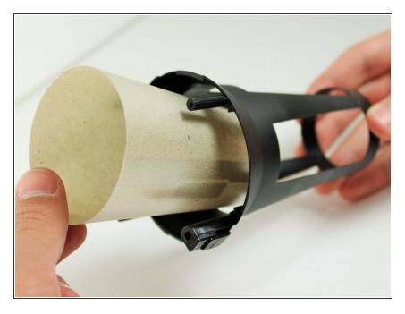
• Gently pull the heat shield out of its sheath.
