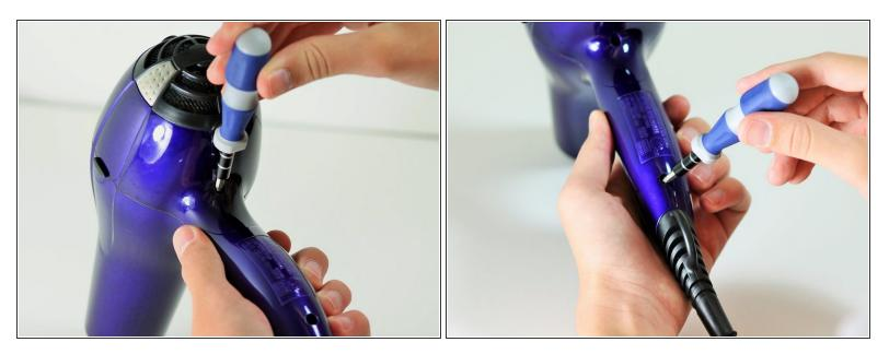
• Remove the two 15.875 mm Phillips #2 screws from the back panel.
