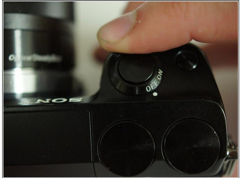
**!** We need to turn off the camera because we are removing components that could get damaged if the power is still on.
