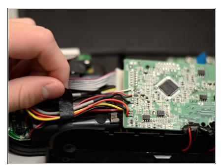
Peel away the tape holding down the wires between the main board and the DC power and 3.5 mm audio jack board.
