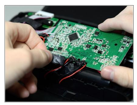
Remove the black tape holding down the four wires connecting the main board to the upper half of the device.
