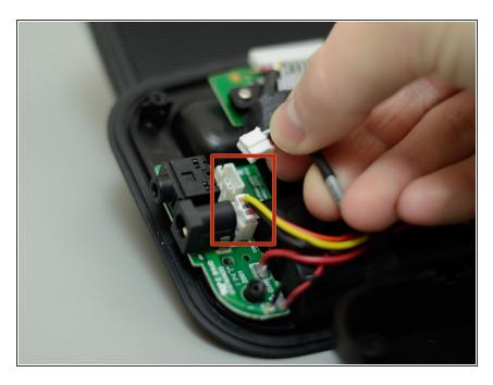
Remove the two 3-pin connectors from the DC power and 3.5 mm audio jack board.
