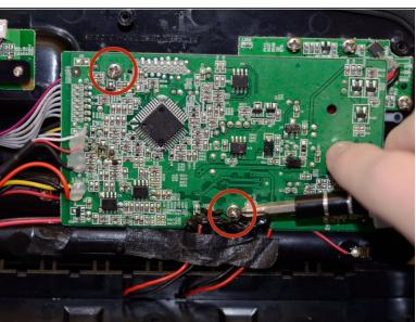
Remove the two 9 mm screws that hold the main printed circuit board onto the rest of the iP37; you will need a Phillips #2 driver to do this.
