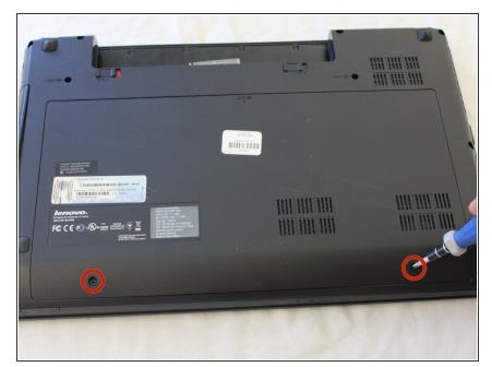
Remove the two screws highlighted.
