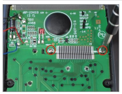
• Next, use a Phillips #00 screwdriver to remove the two screws located on each side of the striped ribbon between the two green circuit boards.
