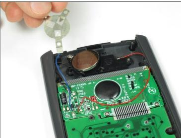
• Use a Phillips #00 screwdriver to remove the two 7.5 mm screws holding the battery cover to the case.
