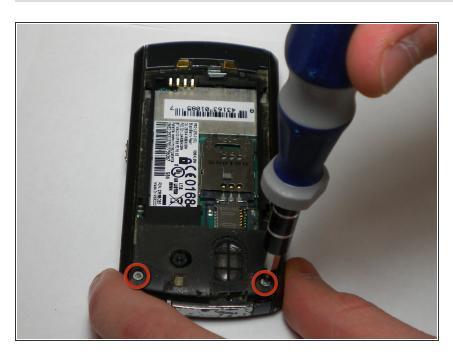
Using a 1.5 mm Hex screwdriver, remove the two screws that hold the two panels together.
