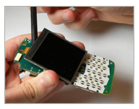
After removing the logic board, place spudger between the logic board and screen and remove the screen, sliding it slowly away.
