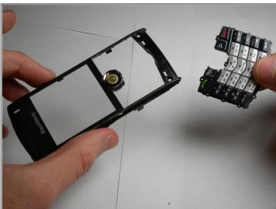
Gently remove the keyboard from front casing. It should snap out of place.
