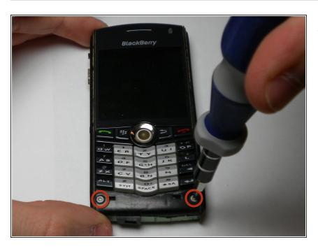
Using a 1.5mm Hex screwdriver, unscrew the two screws, located on the front of the phone, that connect the back and front panels.
