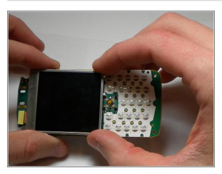
To place the screen on the new logic board, place the goldencolored filament in the slot above the screen's position, similar to how the old one was placed. There are two pegs that fit into the logic board and secure it.
