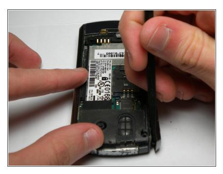
Using the spudger, pry off the side casings one at a time by wedging it between the inner casing and the sides.
