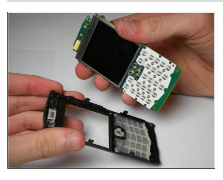
Separate the logic board from the front panel.
