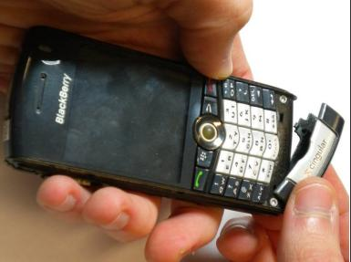
• Using the spudger, pry off the small portion of the casing located at the bottom of the phone.
