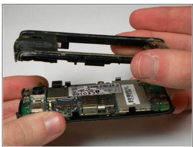
Using the spudger, pry off the back body panel by wedging the spudger in between the front and back panels on the side face. Remove the back body panel.
