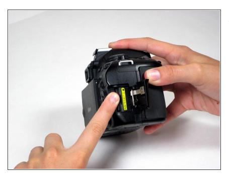
Eject the memory card by pressing it into its slot until you hear a soft "click."
