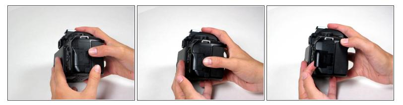
• Open the memory card compartment door, located to the right of the digital display, by using your thumb to push it in the direction of the arrow.
