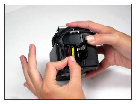
• Using thumb and forefinger, gently remove the SD card from its slot.
