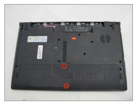
Locate and remove the two 5.3 mm
