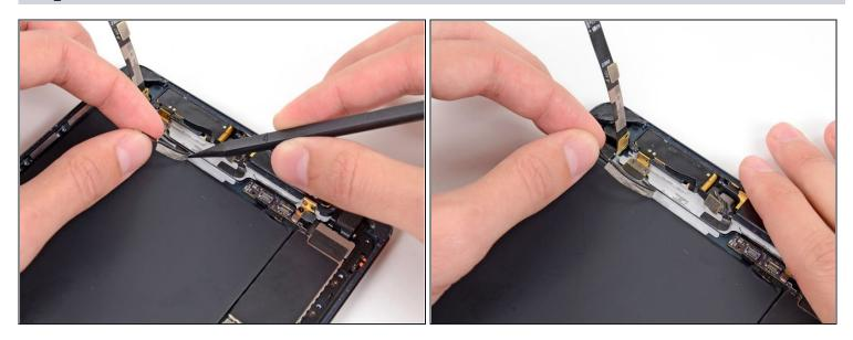
• While gently pulling up on the top left antenna cable, continue using the tip of the spudger to separate the tape from the rear case.
