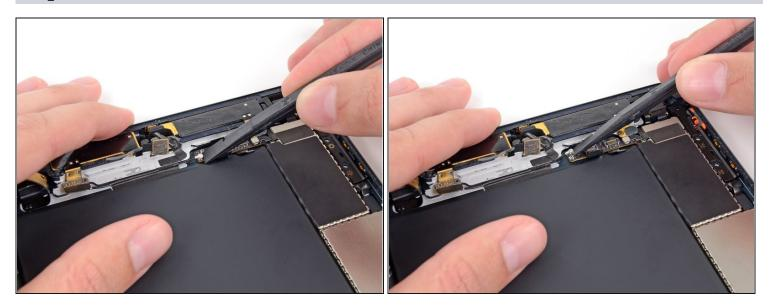
• Use the flat end of a spudger to pry the top left antenna connector from its socket on the logic board.
