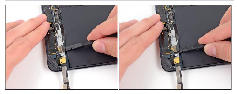
• Slide the flat end of a spudger beneath the top left antenna's screw tab, separating the small bit of adhesive holding it in place.
