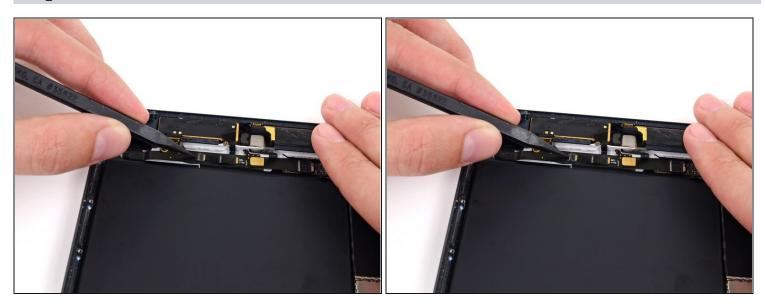
• Use the tip of a spudger to gently lift the tab on the top left antenna ribbon cable's ZIF connector.
