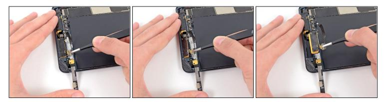
• Use tweezers to lift the top left antenna up and out of its socket in the rear case.
