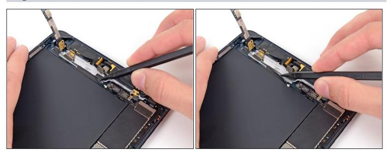
• Use the tip of a spudger to peel back the tape securing the top left antenna cable to the rear case.
