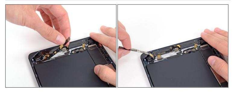
• Lift the headphone jack cable up and fold it out of the way.
