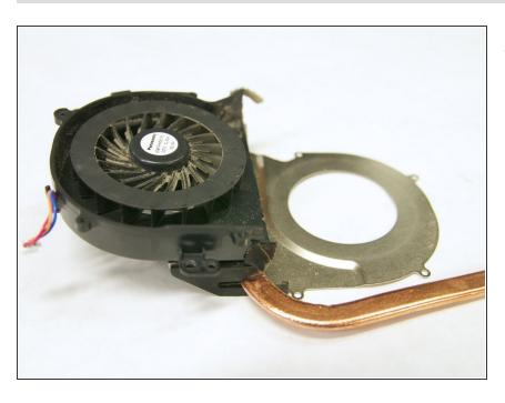
The fan attached onto the heat sink with electrical tape. Removing the electrical tape allows you to replace the fan.
