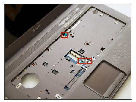
Remove the highlighted ribbon cables from their place underneath the keyboard. To do so, lift up on the black clamps to release the cables.
