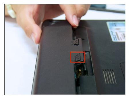
Push and hold the right-hand switch, which says "release" above it, and lift the battery up out of its place.
