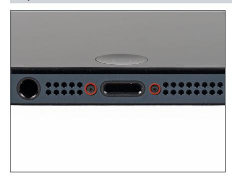
Use the Pentalobe screwdriver to remove the two 3.6 mm
