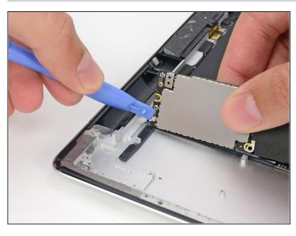
Use a plastic opening tool to disconnect the right antenna cable from its socket on the communications board.
