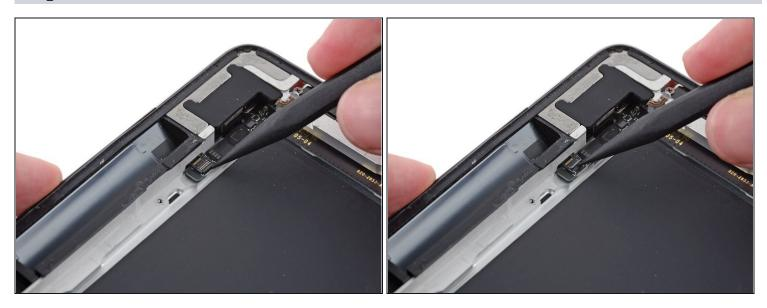
• Use the tip of a spudger to flip the retaining tab on the ZIF connector to release the GPS cable.
