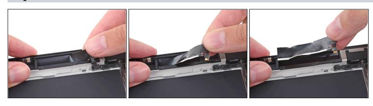
• As soon as you can grip the GPS antenna with your fingers, peel it up off the rear case to remove it.
