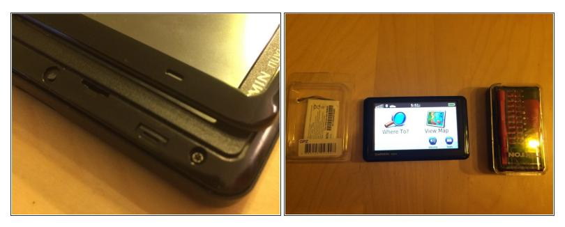
• When you replace the decorative bezel, note that there is a small hole in the bezel that corresponds to a hole in the inner bezel.
