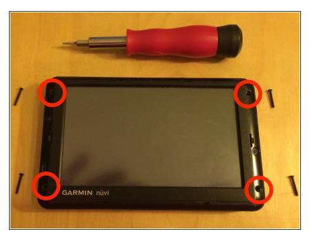
Using your T5 driver, remove the four screws in the corners of the newly-revealed screen bezel.
