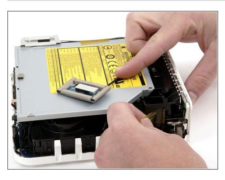
Remove the yellow tape securing the power button cable to the black plastic framework.
