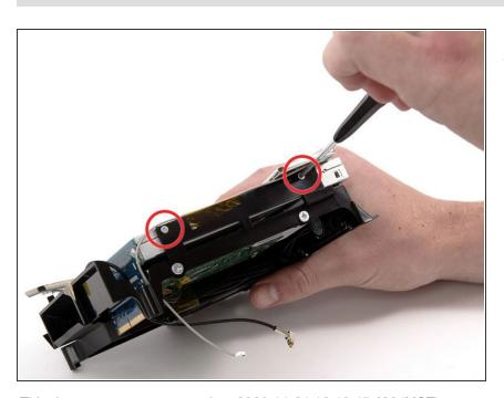
Remove the four silver Phillips screws attaching the optical drive to the black plastic framework (two on each side).
