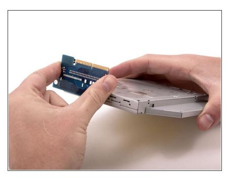
Grasp either side of the interface board and wiggle it free of the optical drive.
