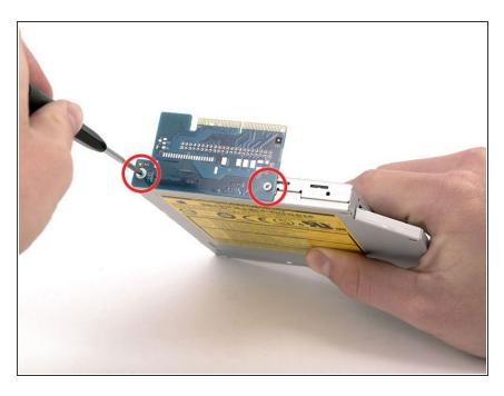
Remove the two silver Phillips screws connecting the interface board to the optical drive.
