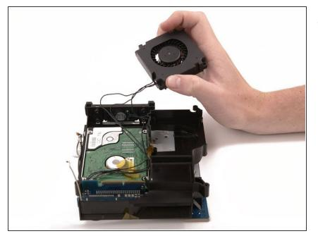
• Lift the fan up and deroute its cable from the plastic framework and the bottom of the hard drive, removing tape as necessary.
