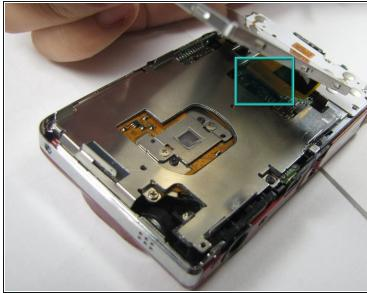
Gently lift up on the left side of the LCD and slowly pull it to the left side of the camera but do not remove entirely, there is a ribbon connector.
