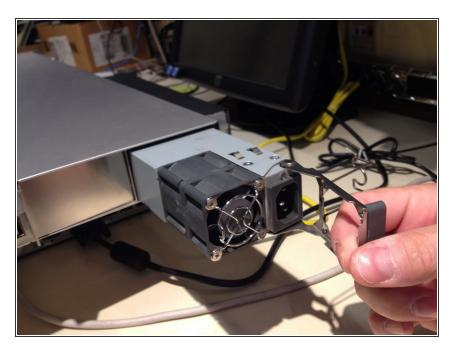
Pull on release lever, and pull power supply out.
